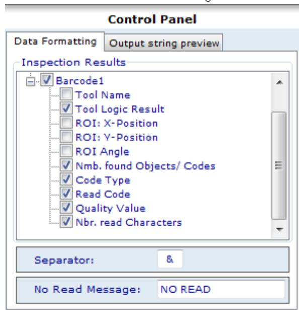
Only selected parameters (check marks) are sent in the inspection result over the RS232 interface. The parameters may be selected or deselected with the mouse individually or by tool.
