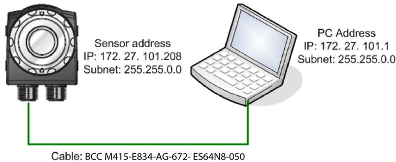
Fig. 3-8: Direct connection of the sensor
