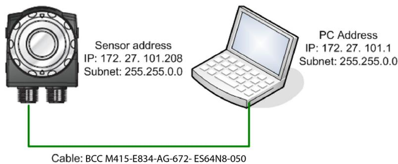
Fig. 4-2: Direct connection of the sensor
