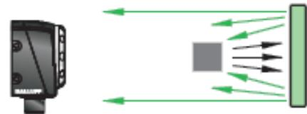
Typical applications include sorting of objects by shape and dimensions, measuring distances between chip connection pins, checking objects for holes or cracks.
