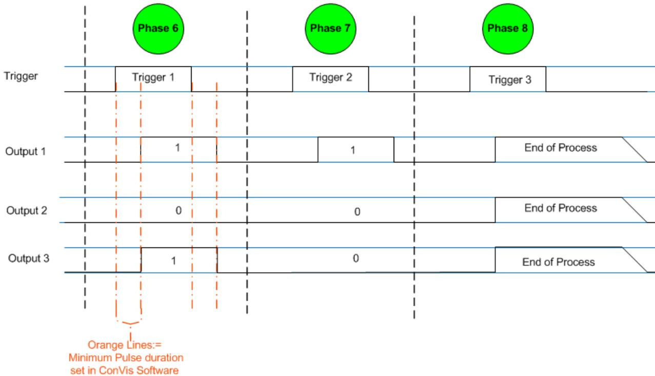
Fig.11-2: Detailed timing diagram for reply, Phase 6 to 8
