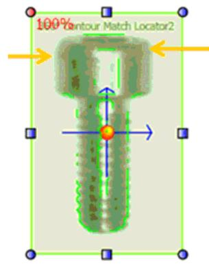
3.) Use the mouse to remove other unimportant contours. Placing the mouse pointer over a selected or deselected contour will show it in yellow.
