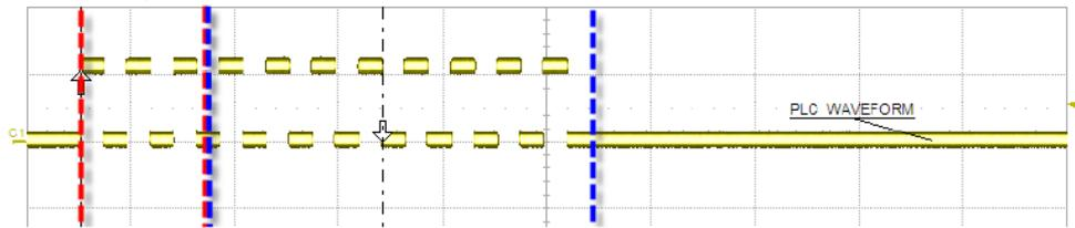
The region between the dashed blue lines contains the data pulses; here you can count 8 pulses, i.e. Inspection Number 8 is being selected.
