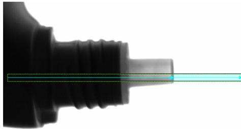
Fig. 8-4a Position checking of the spout of a dish liquid bottle: **OK**
