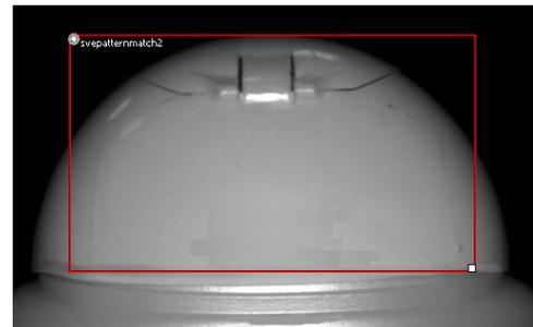
Fig. 8-3b Pattern detection of a shampoo bottle seal: NOK
