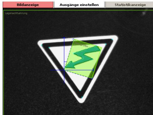
An incorrectly printed label is found, but its actual value is significantly lower (here approx. 65% compared with 90% otherwise) and is therefore detected as **NOK**.
