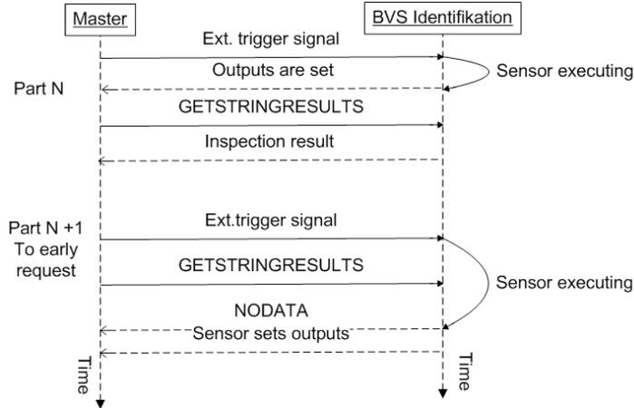
Fig. 9-2: Synchronous communication
