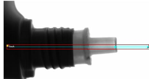
Fig. 8-4b Position checking of the spout of a dish liquid bottle: **NOK**
