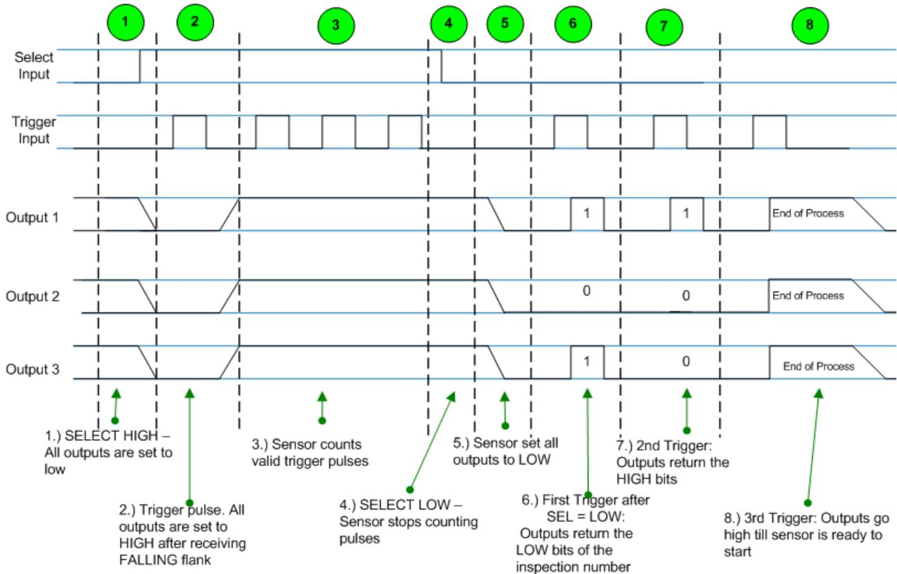
Fig.11-1: Timing diagrams Phase 1 to 8
