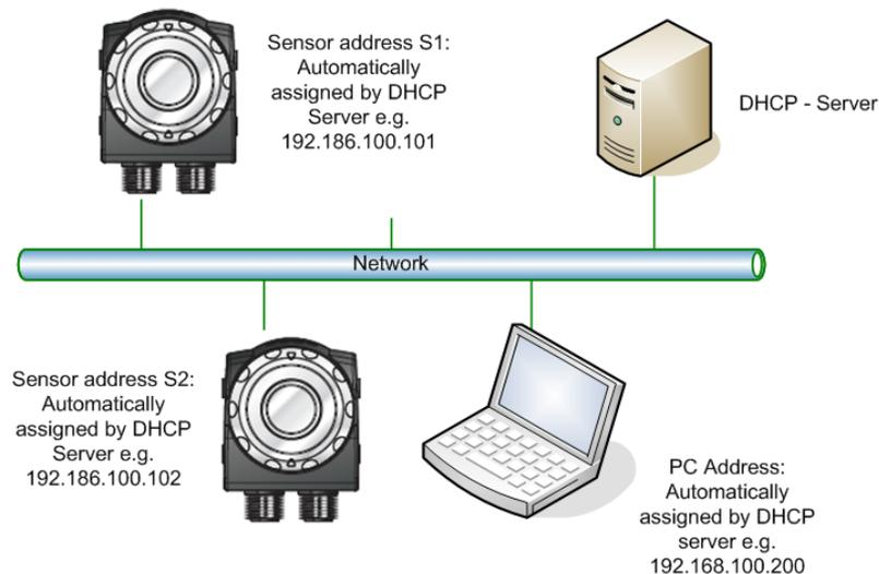
Fig. 4-3: DHCP connection of the sensor
