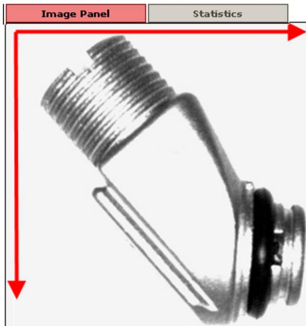
This means that if the part in the current image is displaced compared with the part in the reference image, the position of the tool ROIs does not follow the part. As a consequence the part may not be correctly inspected.
