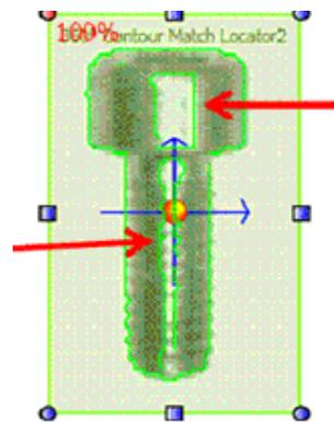
Be sure when changing the Noise Suppression parameter you do not remove any contours important for the inspection, e.g. on the screw head.
