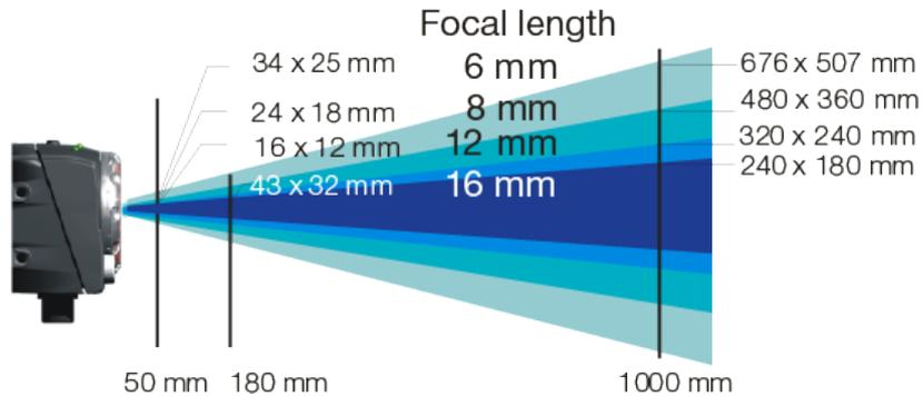
Fig. 16-5 Field of view for sensor models
