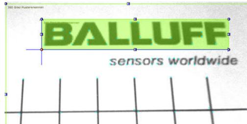
If this feature is rotated 90° clockwise, for example, then the alignment of the logo changes also. There is no longer agreement between the reference pattern and the detected pattern.
