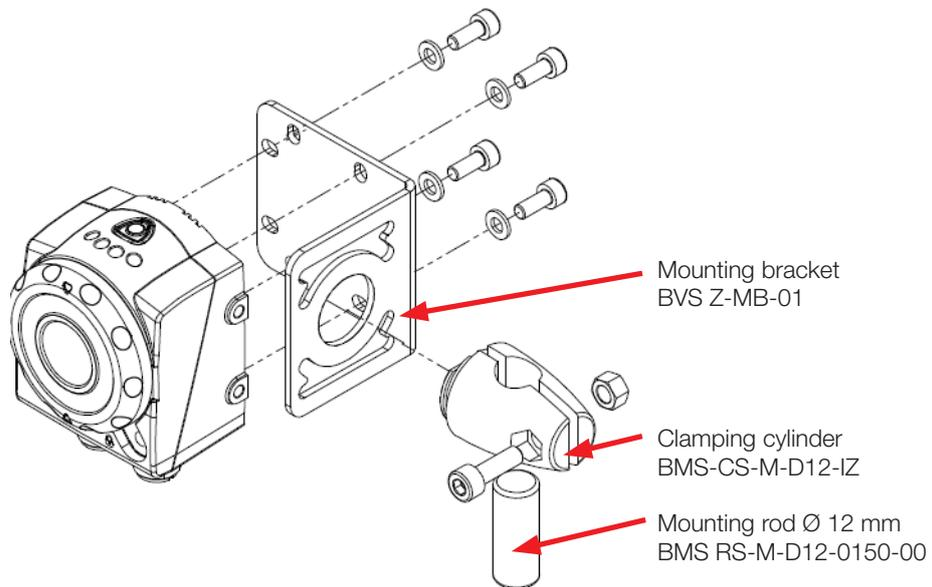
Fig. 3-3: Sensor attachment using mounting accessories
