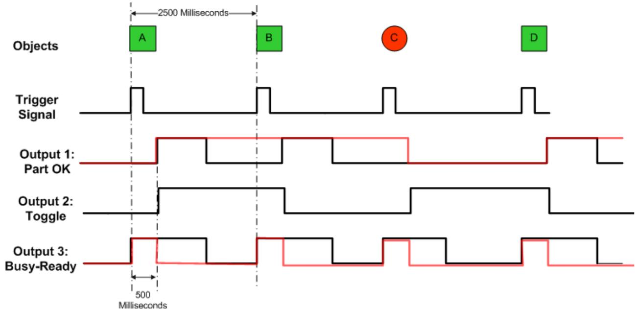
Fig. 10-3: Diagram for output timing
