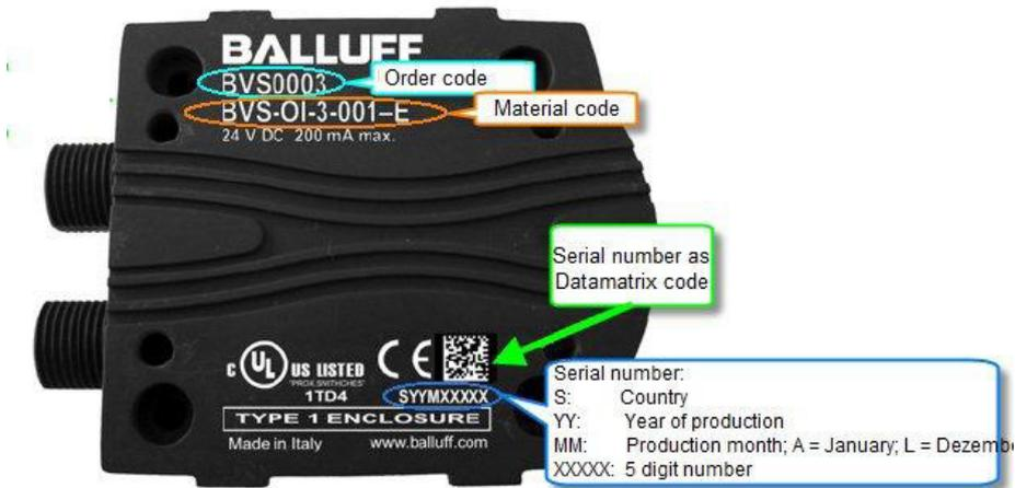
Fig. 16-1 Sensor type identification
