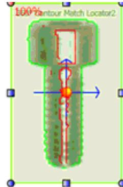
You can also remove ALL contours by clicking on the corresponding button in the field. Then you can use the mouse to add individual contours by left-clicking on the red lines.
