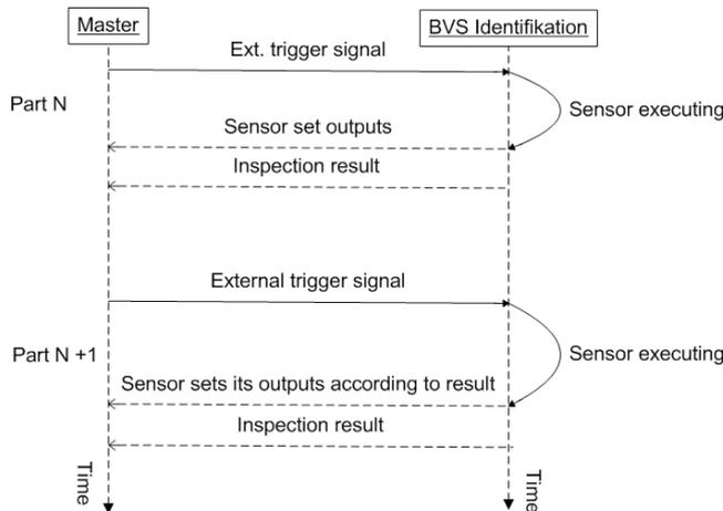
Fig. 9-3: Asynchronous communication
