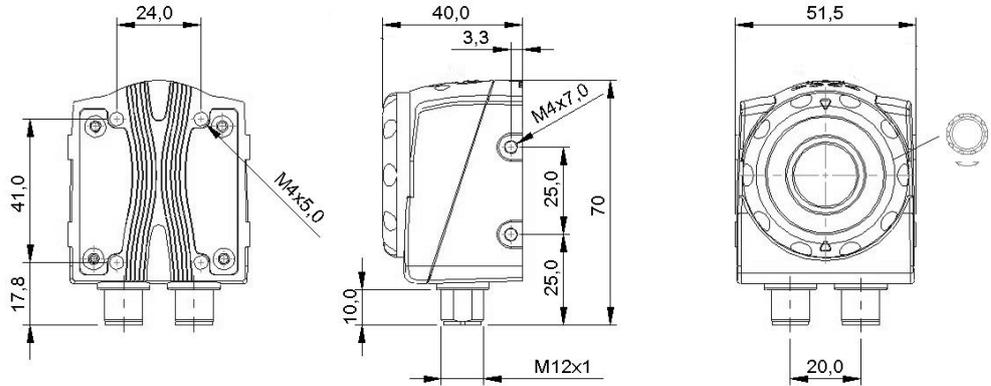
Fig. 16-2: BVS-E, dimensions (in mm)
