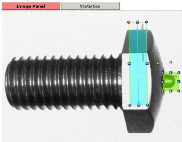
Now enlarge the ROI of the tool - the position change of the part must always take place within the ROI, otherwise the position cannot be located. Now adjust the permissible Maximum to your application. As the position of the part changes as in the following illustration, the "edge" of the head is found and the tool is located.
