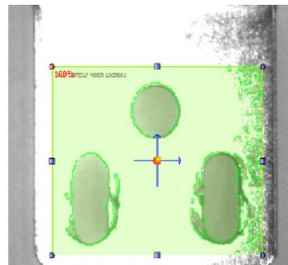
In this case we recommend setting the brightness and contrast (Step 1) differently and if possible changing the alignment of the sensor to the part. Also, the use of external lighting may provide dramatic improvement.
