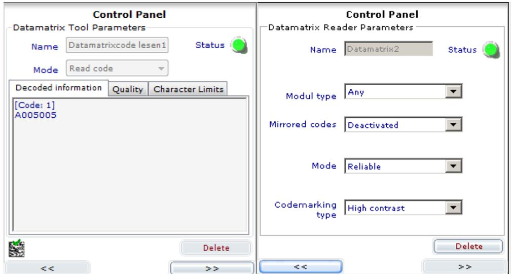
Fig 8-15: Control panel for Read Data Matrix, page 1 and page 2
