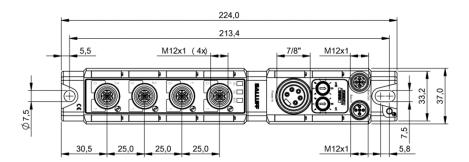
The BNI PBS-... module can be connected directly to a mounting wall or to a machine. Be sure that the mounting base is flat to prevent any mechanical stress on the device housing.
