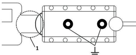
The narrow area (1) between the measuring electrode and electronics box is an electrically and mechanically sensitive area. Moisture in this area can affect the measurement value.
