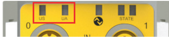
Figure 5: Position of the LED indicators for US and UA
