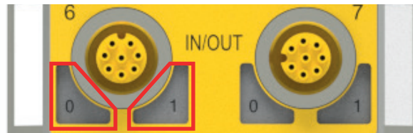
Figure 13: Position of the LED for a multi-function port (Port 6 shown here)
