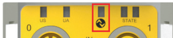
Figure 7: Position of the IO-Link LED
