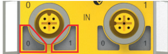
Figure 9: Position of the LEDs for an input port (Port 0 shown here)
