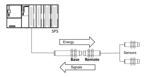
The BIC system transmits two binary sensor signals from the mobile unit (remote) via the air gap to the stationary unit (base). In addition to this signal transmission, the BIC system provides electric power to the sensors connected to the remote.
