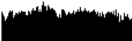
Fig. 3-7: Light band incorrectly aligned, left edge of the CCD not illuminated
