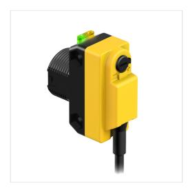
WORLD-BEAM QS18 Series: Polarized Retro Range: 3.0 m; Input: 10-30V dc Output: Complementary Solid State NPN 2 m (6.5 ft) Cable Part Number: 87384
