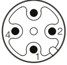
Fig. 4-4: Pin assignment of S4 connector (view from above on connector of BIP)
