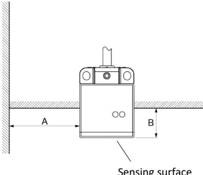
The diagram shows a single inductive coupler mounted on a metal surface. Dimension 'A' is the lateral distance from the metal surface to the sensing surface. Dimension 'B' is the distance from the sensing surface to the rear mounting surface. The sensing surface is marked with crosshairs.
