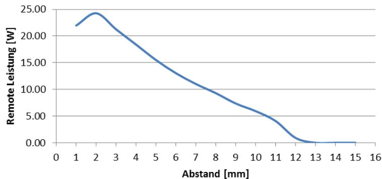
Derating curve: output power of the Remote at 24V-5%
