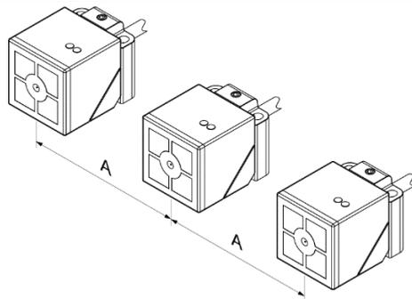
The diagram illustrates three inductive couplers mounted in a row. Dimension lines labeled 'A' indicate the minimum lateral distance between the sensing surfaces of adjacent units.
