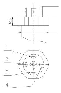
Output 4 to 20 mA, power supply from the current loop:
