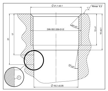
1: Rtmax 6.3 must be guaranteed in this area, as the sealing ring is located here!
