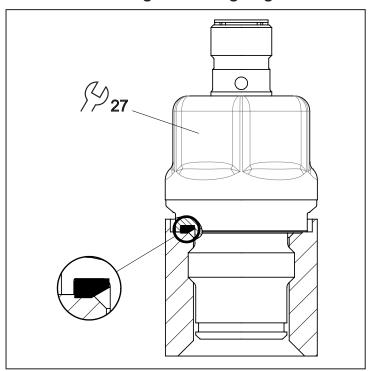
The rear sealing ring made of FKM according to DIN EN ISO 1179-2 (order no.: E30492) has extended chemical resistance and is factory-mounted. Further moulded seals made of FFKM (order no.: E30513) and EPDM (order no.: E30451) are available as accessories.
