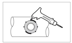
Fig. 4: Applying the fixing points
