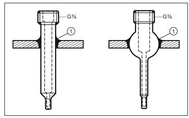
Fig. 3: Installation according to EHEDG with welding thermowells
