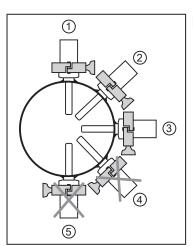
Fig. 1: Installation position for 3-A certification
