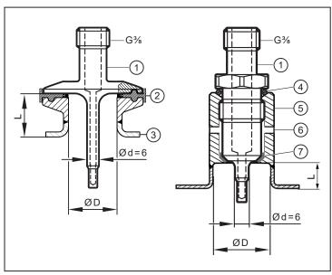
Fig. 2: Mounting dimensions for EHEDG approval
