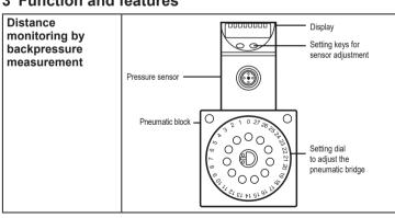
The system monitors whether distances from 10  $\mu$ m to approx. 400 $\mu$ m (max. approx. 700 $\mu$ m depending on the number and diameter of the backpressure nozzles and the measurement situation) are adhered to / exceeded.
