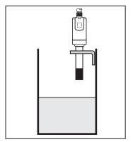
Empty the tank until the medium is at least 20 mm below the end of the probe.
