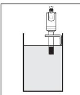
Fill the tank until the active zone is completely covered.
