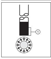
The device operates with radial detection characteristics. Therefore, media below the active zone (1) are not detected.
