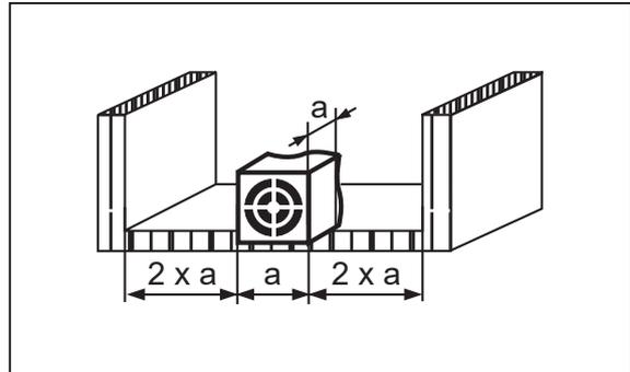
Fig. 5: rectangular design, non-flush
