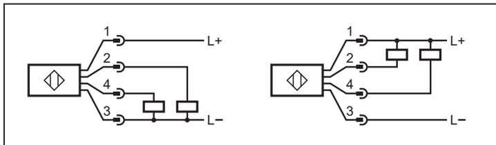
Fig. 9: example connection PNP/NPN
