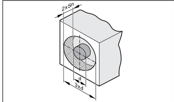
Fig. 3: cylindrical design, non-flush
