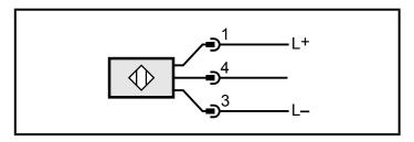
Pin 1 = L+ (10...30 V DC) Pin 3 = L-Pin 4 = IO-Link (Pin 2 = not connected)
