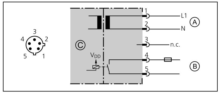
A: supply circuit; B: output circuit
