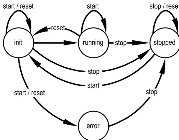
After the initialisation in the "init" state has been completed, the connection automatically changes to the "running" state.
