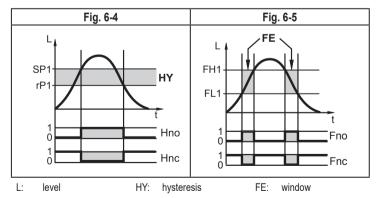
For the switching output a switch-on and switch-off delay of max. 60 s can be set (e.g. for especially long pump cycles); ( $\rightarrow$  10.4).
