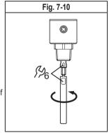
In case of high mechanical stress (strong vibration, moving viscous media) it may be necessary to secure the screw connection, e.g. by a screw retaining compound.
