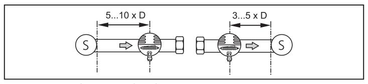
D = pipe diameter; S = sources of interference
