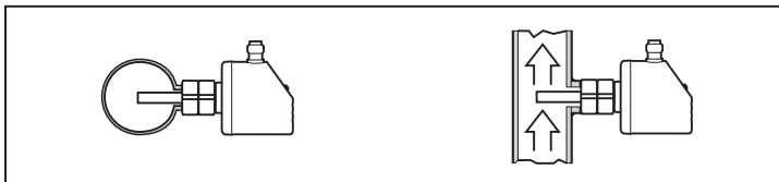
Fig. 6: Recommended mounting position
