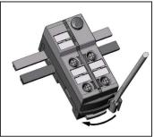
Open the unit using a tool as shown (e.g. screwdriver).
