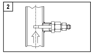
Components integrated in the pipes, bends, valves, reductions, etc. lead to turbulence of the medium. This affects the function of the unit.
