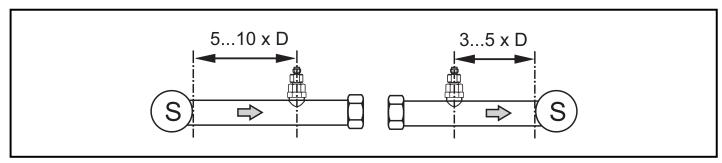
D = pipe diameter; S = sources of interference
