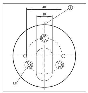
Fig. 1: Fixture (view from bottom)
