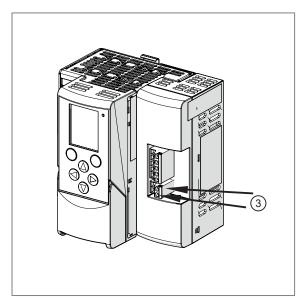
3: 3: Total supply from an AUX power supply or an AS-i power supply
