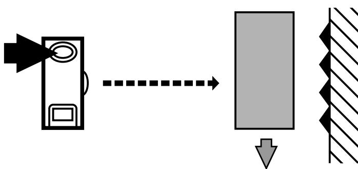
The yellow and green LEDs go out for approx. 1s, after approx. 3s the green LED is on.
