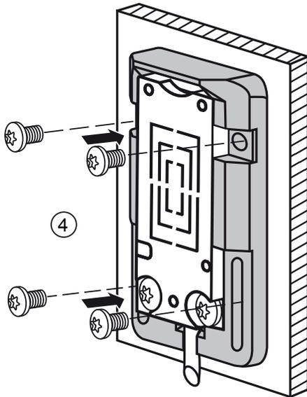
Fig. 3: Attach the mounting adapter to the tank
