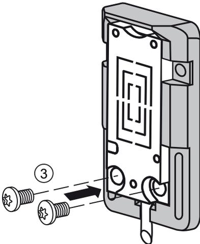
Fig. 2: Attach the device to the mounting adapter
