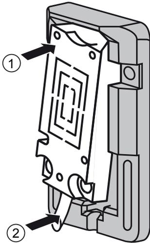
Fig. 1: Insert the device in the mounting adapter
