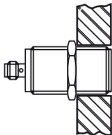
Fig. 3: Flush mounting
