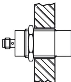
Fig. 4: Non-flush mounting
